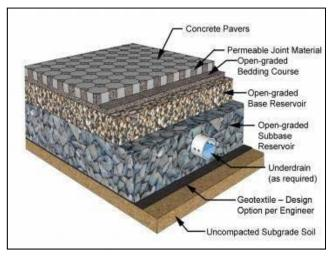
Pervious pavement is designed to allow percolation or infiltration of storm-water through the surface into the soil below where the water is naturally filtered, and pollutants are removed.
